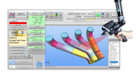
This is the software tool designed exclusively for **tube measuring, tube-shape qualification, tube bender correction,** and **tube-shape reverse engineering** using laser scanners.
