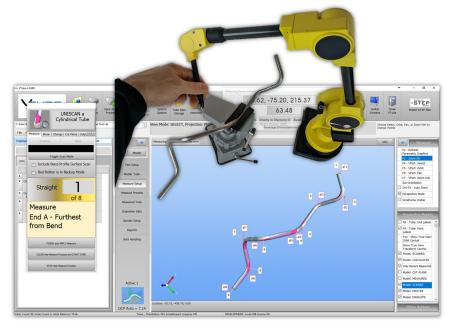
This is the software tool designed exclusively for tube measuring, tube-shape qualification, tube bender correction, and tube-shape reverse engineering using touch probe technology.
